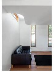
No artifical light is needed during daylight hours in this new house in Eitham, Victoria, designed by Lume Architecture. No part of the house is more than four metres from a window, and in many rooms windows face different directions to allow for natural light throughout the day.
